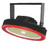
LED HIGH BAY: Advance ergonomic light distribution, high transmittance lens for even light distribution. The LED highbay is available in four optical beams for different type of wattages (100W / 120W / 150W / 200W). 100V - 240V at 50 000 hr rated life expectancy. Operates at -30°C ~ + 50°C. Luminous Efficacy 140lm/W. IP65.
