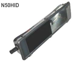
ZONE 2 CORROSION RESISTANT: Available in 304 and 316 marine grade stainless steel. Luminaire range has a deep drawn stainless steel body, single piece pressed frame and stainless steel clips. The 4 mm thick lens is clear armour plate glass. Mounted on a gear tray, comprising the 150W HPS choke, Power Factor correction capacitor and ignitor with thermal cutout which protects the choke, and prevents the possibility of sparking during lamp change. IP65.
