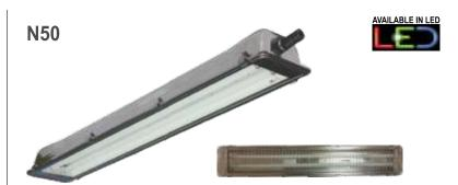
**ZONE 2 CORROSION RESISTANT:** Available in 304 and 316 marine grade stainless steel. Luminaire range has a deep drawn stainless steel body, single piece pressed frame and stainless steel clips. 4 mm thick clear armour plate glass. Electronic Control Gear and LED driver are approved for Zone 2 applications. Available in single and double lamp 18W, 36W and 58W versions. Lens wire guard is available as an optional extra. **IP66**.
