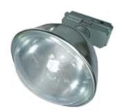
ZONE 2 HIGHBAY: control gear housing in GRP Suspension hooks carry the weight of the luminaire. Die cast aluminium lampholder assembly. 4 mm thick armour plate glass with polycarbonate shield spun into the polished reflector. Applications: Food industry, Tissue Production. IP66.
