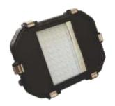
LED ZONE 2, 21 & 22 Luminaire: High Pressure Die Cast Aluminium body and frame supplied with stainless steel clips. 4mm thick clear armour plate glass. The LED modules and control gear are approved for Zone 2, 21 & 22 applications. Circuit watts from 35W to 150W. IP65.
