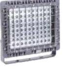
Series BLD150LED Nordland Ex-Proof floodlight are for use in locations such as Zone 1, 2, 21 & 22. Ex Protection: Ex d IIB T6 Gb / Ex tb IIIB T85°C Db IP65 Circuit watts 20W to 160W; > 50 000 hr rated life expectancy. IP 65
