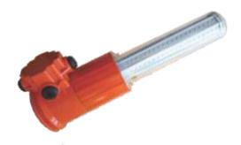
For Zone 1 group I/IIB T6 to be used underground and surface coal mines. Applications: Walkways; Conveyor belts; Roadways etc. Fluorescent tubes: 600 mm, 1200 mm and 1500 mm avaliable; Compact fluorescent energy savers and LED options. Clear flame retardant polycarbonate lens cover: 110V – 220V; 12V, 24V and 36V.
