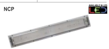
**PRISON FITTING:** Heavy duty luminaire based on the JB Polycarbonate diffuser with sheet steel fabricated body and lens frame. Available in 304 and 316 marine grade stainless steel. Also available in galvanised steel. Require a special tool to open luminaire. 1,2 mm thick clear polycarbonate lens, with internal linear prism to limit glare. Sealed into the fabricated frame. The combination is designed for impact strength, and appearance. **IP 54.**
