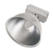
HIGHBAY: DMC glass fibre reinforced polyester, compression moulded in two sections. Control gear housing in GRP. Suspension hooks carry the weight of the light fitting during installation. IP 20.
