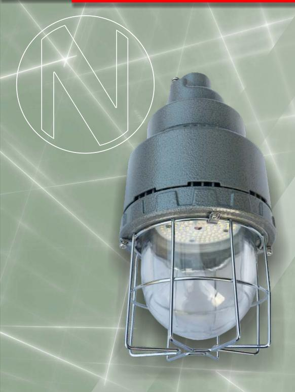
The **HA1** is a high performance LED pendant luminaire, designed and certified for Zone 1, 2, 21 and 22 hazardous areas. The luminaire is designed to replace the conventional HID lamp technology which makes it energy efficient with high performance, low maintenance and long life span. It's suitable for wall, ceiling, pendant and pole mounting. The **HA1** continues the proud heritage of NORDLAND LIGHTING's Ex safety standards whilst utilizing the latest LED technology.
