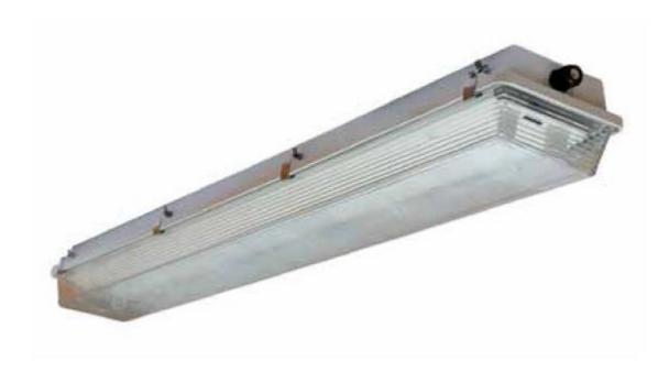
**JBF- LT** is a range of enclosed corrosion and vapour proof luminaires, has a flame retardant body polycarbonate injection moulded lens with linear prisms and stainless steel clips. Are available in 600mm; 1200mm and 1500mm T8 **LED** tubes. The luminaire is dust and moisture proof, making it ideal for applications such as indoor car parks, warehouses, dry and cold storages.
